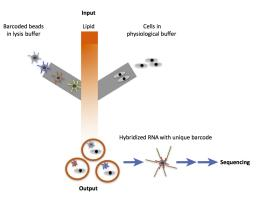
A single device has three input ports (oil, barcoded beads in lysis buffer, and cells of interest) and a single output port used for collecting bead-cell-containing lipid droplets. Then each cell (or RNA in the cell) is marked by the unique barcode and processed on the bead for sequencing
